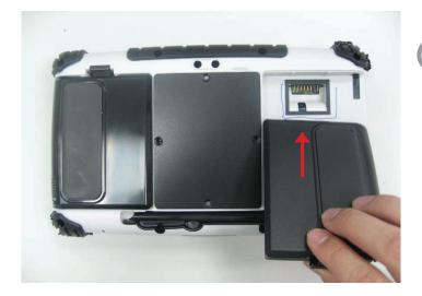
Insert the battery pack into the battery slot.
