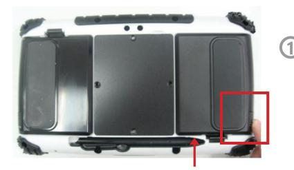
Slidethe latch up to release the battery cover
