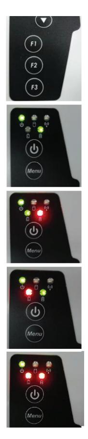
c. Give a long push to the <F3 > button to switch the discharging status between left and right battery
