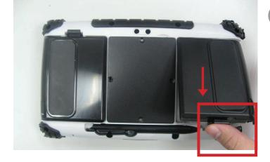
Press down the compression lock into the tablet pc.
