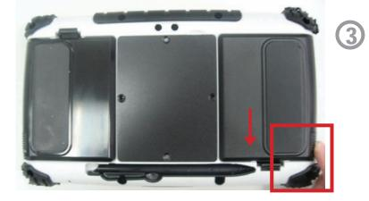
Press the latch down to fasten the battery on the tablet PC
