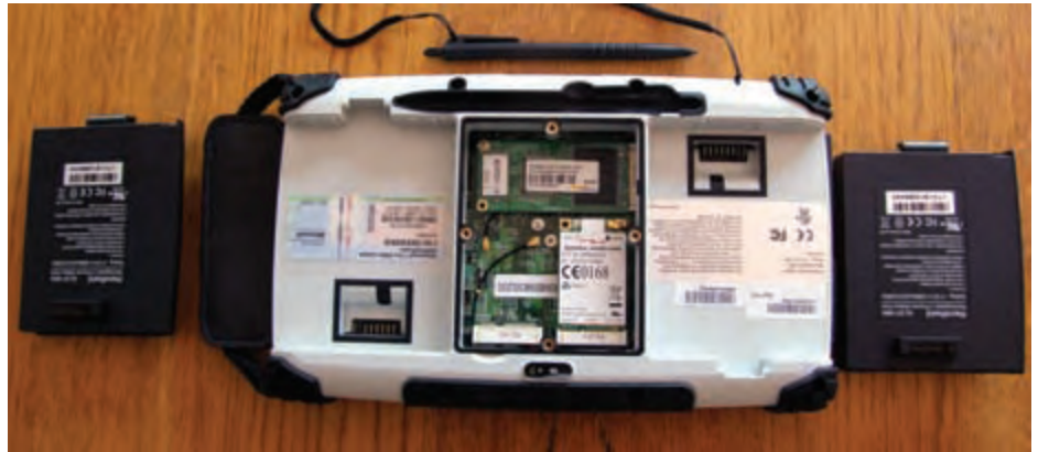
The Algiz7 with the batteries in place and removed, with the motherboard exposed.
