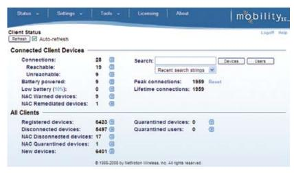
The "Client Status" tab shows device connectivity status, number of quarantined devices and even battery life. From this screen, administrators can search for information on a specific user or device, such as open applications, device operating system and interface or port in use.
