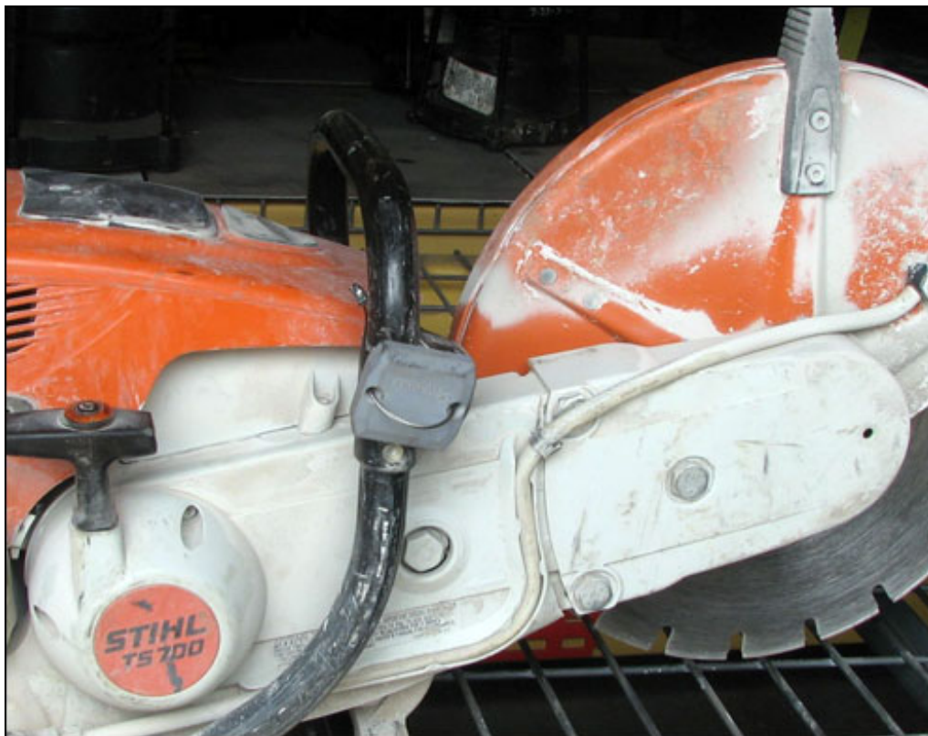
For tools that are used outdoors and exposed to rough treatment, Seminole County utilized RFID tags designed to be especially rugged.
